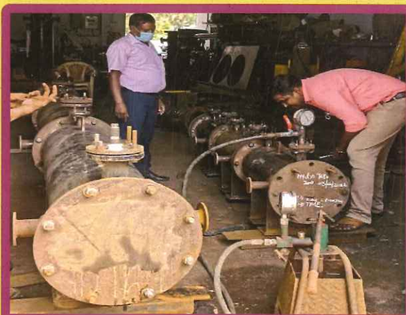
ALL TYPE OF FABRICATION & HYDRO TEST 13 BAR
