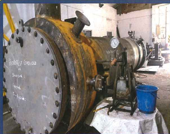
ENTIRE SHELL HYDRO TEST
