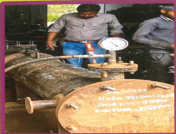
300 SHELL HYDRO TEST
