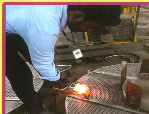
DISSOLVING BASKET SS316 L GRADE PMI TEST IN M/s.MICRO LAB
