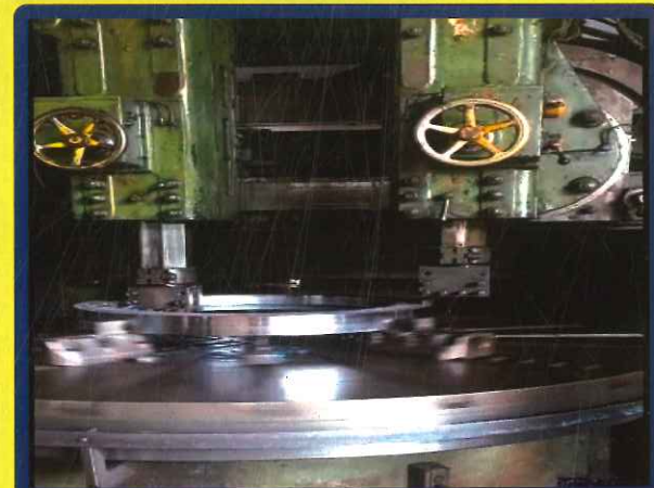
CNC VTL LATHE FLANGE MACHINING UPTO 5 MTRS
