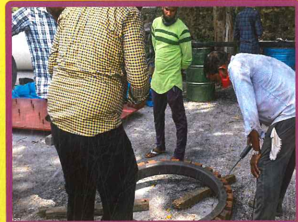
RUBBER LINING SPARK TEST FOR M/s.MIL
